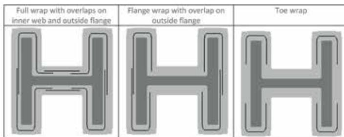
**Potential mesh overlap configurations on a column. The position of overlaps will depend on product specification and size/shape of the column. The overlaps along the length would also need to be considered.**
