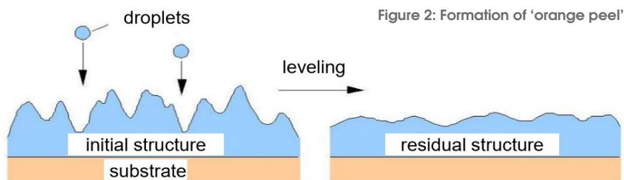
Figure 2: Formation of 'orange peel'
