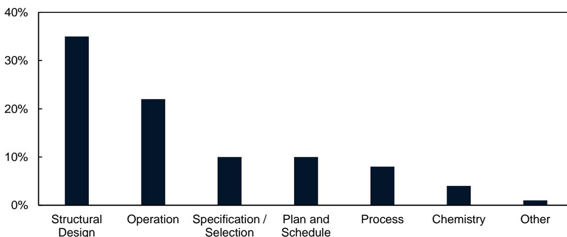
**Figure 1: Main causes of coating failure (%) based on Safinah investigations**
